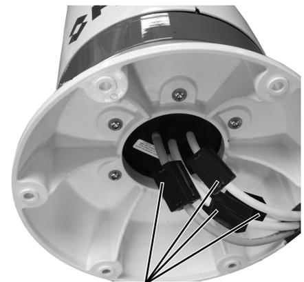
Ferrites installed on cables under top-down riser
