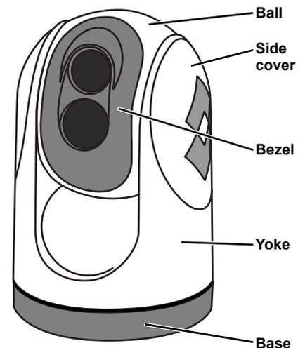
Do not use abrasive materials, such as paper or scrub brushes as this will possibly damage the lens by scratching it. Only wipe the lens clean when you can visually see contamination on the surface. Never use ammonia-based cleaning products on the optics.
