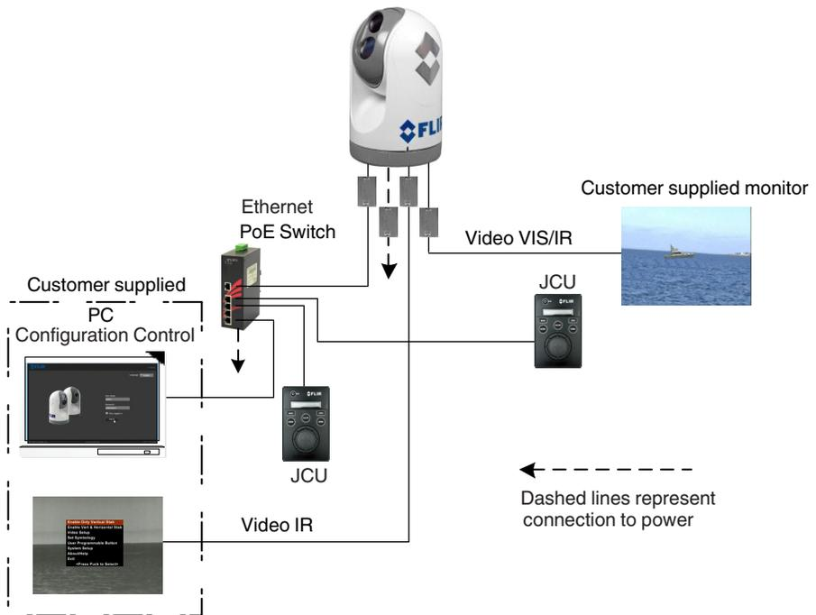
Figure 1-2: Two station installation with a PC
